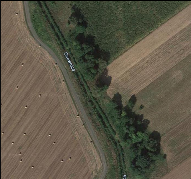
Figure 12: Osownica stream straightened.
