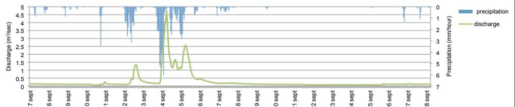
**2** The second graph shows that only a small proportion of the precipitation is discharged immediately, while the river basin as a whole stores an enormous quantity of water.
