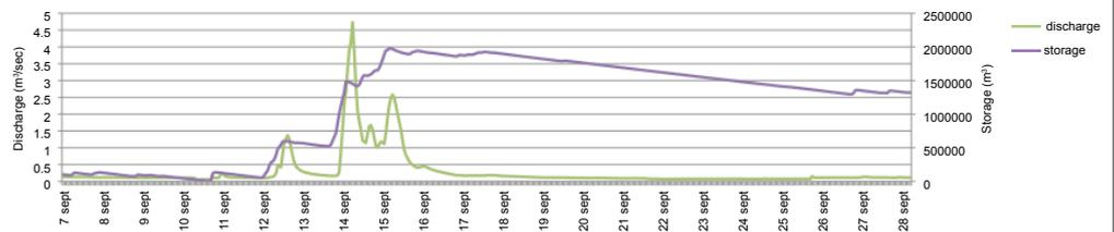
**3** From the third graph it becomes clear that the greatest proportion of the precipitation does not discharge immediately but is buffered somewhere in the sponge within the basin and is released over a longer period of time.
