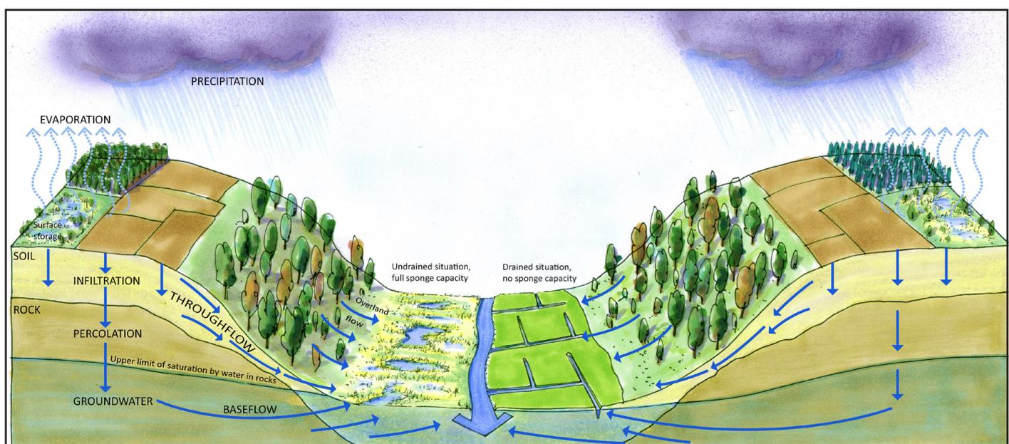
Figure 1. The role of drainage at the foot of the slope. On the right hand side the valley is drained by means of channels, on the left hand side the undrained situation.
